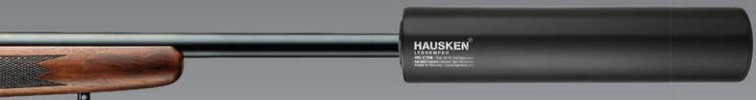
Hausken sound moderators are manufactured in Norway in hard-anodised, high quality aluminium for durability. The moderators have two main parts with the baffles being machined from a solid aluminium bolt, 35mm, 45mm, 55mm or 70mm in diameter. Each moderator is fitted with an 18x1mm thread but, using the unique Hausken barrel nut conversion system, the thread is adapted to suit your rifle.
